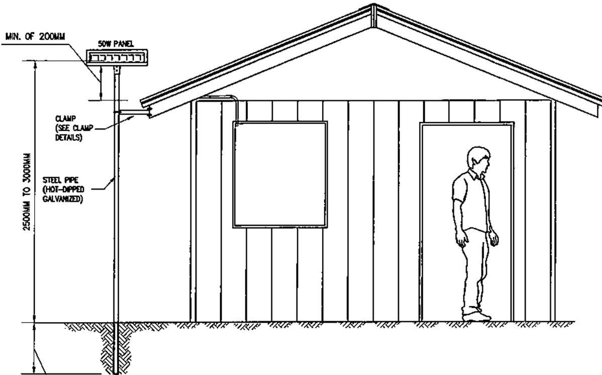
(MIN. DEPTH 500MM) **TYPICAL ROOF SIDE POLE MOUNTED PV MODULE**
