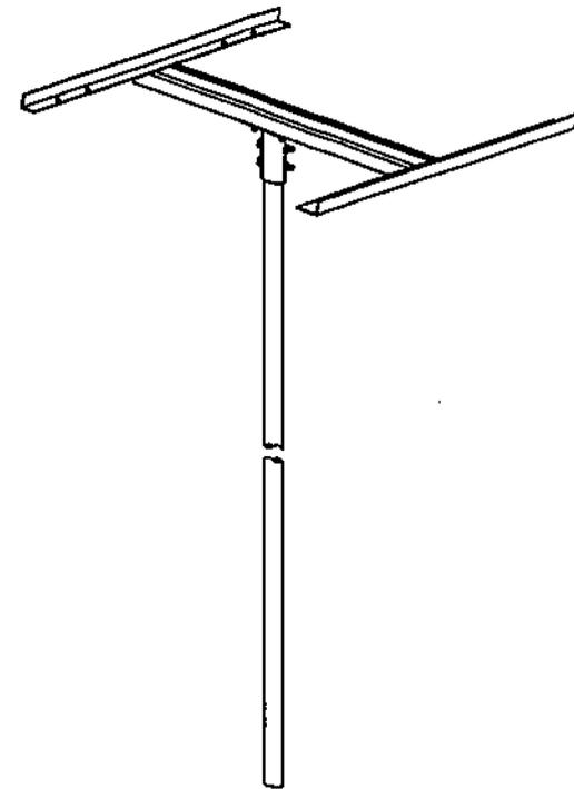
**ISOMETRIC VIEW OF PV MOUNTING PIPE**
